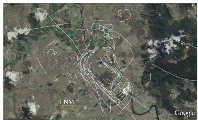
Fig. 15. The short-range radar tracks from Fig. 14 showing aircraft tracks in the circuit (pattern) area.
