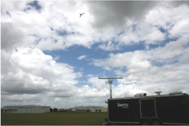
Fig. 1. The Mobile Aircraft Tracking System (MATS) is installed in a trailer that forms part of Insitu Pacific's UAS Flight Demonstration System. The MATS uses a primary surveillance radar and other sensors to monitor the local air traffic. The photo was taken at Watts Bridge airfield during ScanEagle operations.
