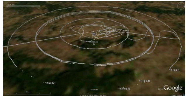
Fig. 10. The ADS-B track of the ASL from 8:24am to 2:10pm on 13 July 2010. The view is to the west towards the MATS. The circular flight paths with radii of 6, 10 and 14 NM from Watts Bridge are easily distinguished. The ADS-B signal was lost whenever the ASL flew into a radio wave shadow region.
