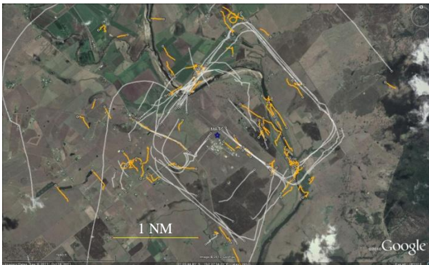
Fig. 16. The primary radar tracks observed from Watts Bridge airfield from 2:12pm to 3:31pm, 13 July 2010. A symbol was used to mark the end of each track and the associated 'tail' shows the track's history. The tracks with orange tails had mean speeds of less than 30 knots.
