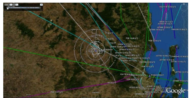
Fig. 12. The ADS-B tracks of the equipped aircraft in the region around Watts Bridge airfield, from 13 July 2010. The ADS-B track of the ASL is also shown.
