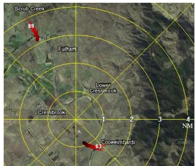
Fig. 3. An example of the MATS real-time radar display, centred on the Watts Bridge airfield. Two aircraft tracks are shown. The aircraft 3.5 NM to the northwest is heading away from the airfield at 89 knots. The aircraft 1.3 NM to the southeast is heading west at 63 knots. Range rings, in one nautical mile increments, are shown.
