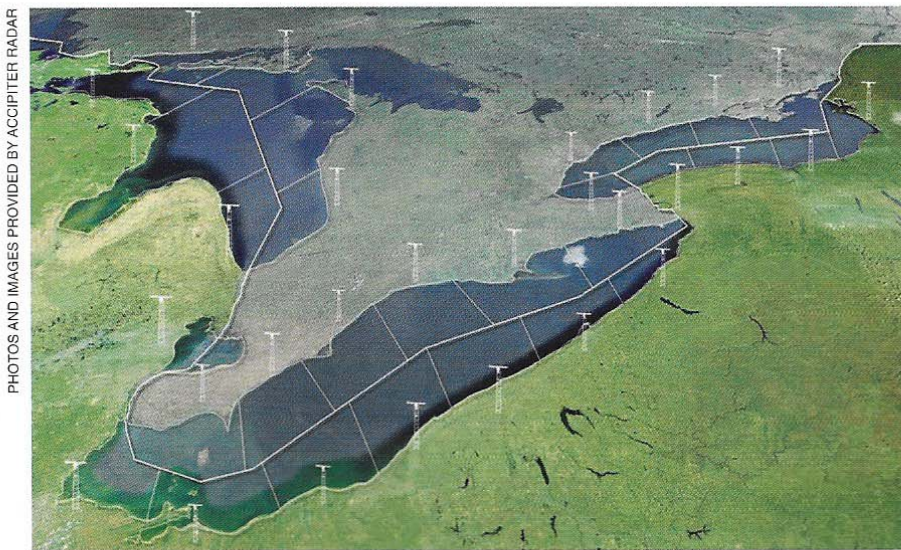
Left: depiction of full-scale, wide-area, radar S2I network on the Great Lakes modelled after cellular networks. Right: photograph of a typical radar node.
