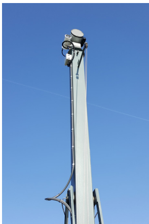
Accipiter® Multi-Device Steerable Platform incorporating high powered acoustic hailing device, thermal camera and high-powered searchlight.
