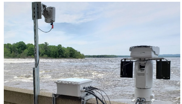
SpotterRF Short Range Radar Sensor with Axis Q8741-LE Bi-spectral Surveillance
