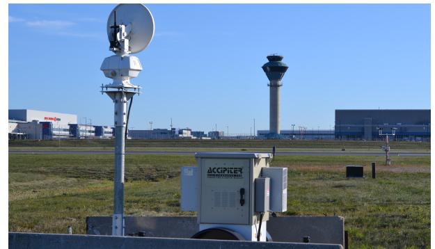
Accipiter® TS1-24D 3D Radar Surveillance System
